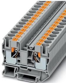
Feed-through terminal block, nom. voltage: 1000 V, nominal current: 57 A, connection method: Push-in connection, Rated cross section: 10 mm<sup>2</sup>, cross section: 0.5 mm<sup>2</sup> - 16 mm<sup>2</sup>, mounting type: NS 35/7,5, NS 35/15, color: gray
